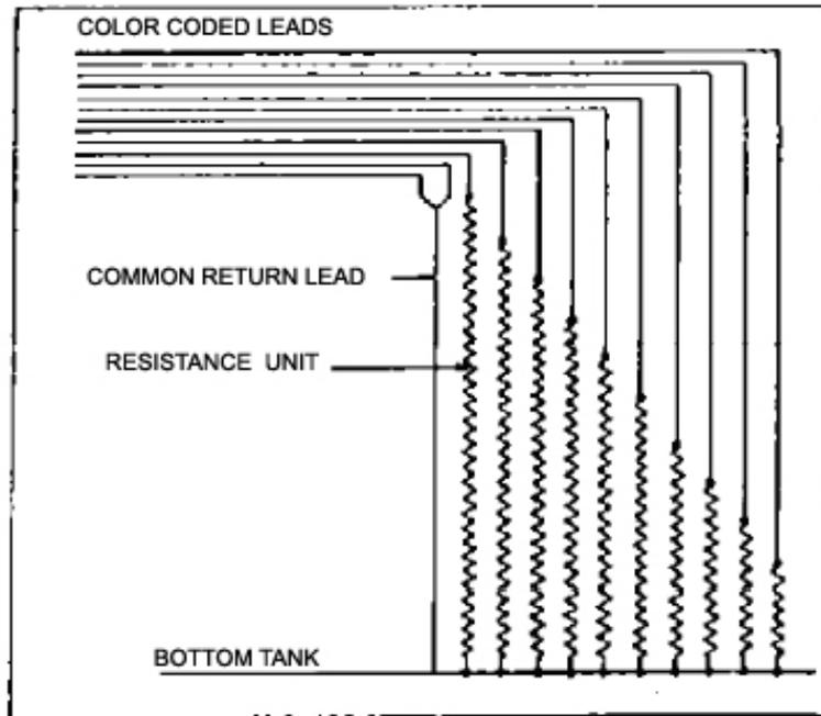
SCHEMATIC DIAGRAM OF AVERAGING-TYPE RESISTANCE BULB
