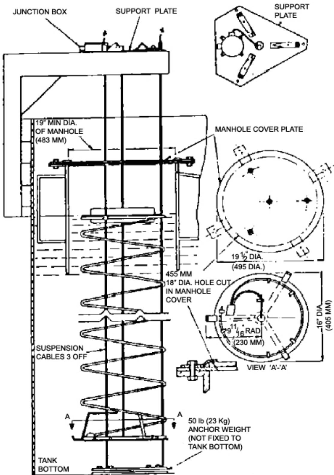
TANK AVERAGE TEMPERATURE RESISTANCE THERMOMETER ELEMENT FOR FLOATING ROOF TANK
